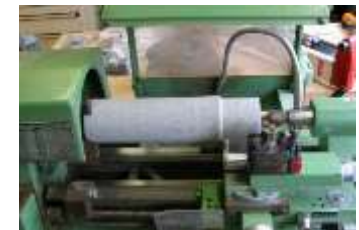
Compacted cylinders bentonite/sand
