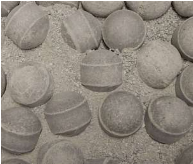
MX80-bentonite pellets-powder mixture
