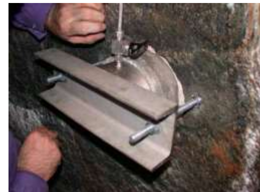
Surface packer system to measure EDZ (BGR)
