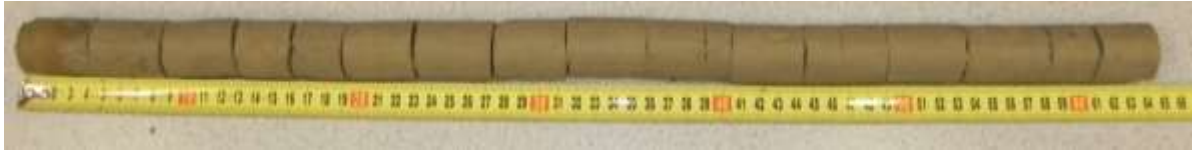
Figure 2 - Core sample of the bentonite barrier extracted by means of vertical drilling
