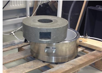
Figure 4. A sketch of the set-up used for the SH1 and SH2 (left) and photos of the test device and the bentonite rings with the cut cavities (right). In the sketch the dimensions of the outer and inner steel cylinders and the bentonite block with the cavities are shown as well as the plastic filters and the locations of the water inlet and outlet (Dueck et al. 2016).
