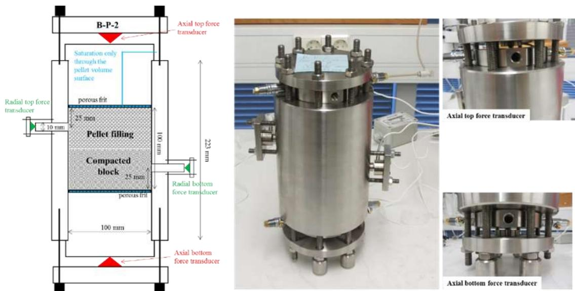
**Figure 5-1** Schematic illustration and pictures of the block-pellet test system.
