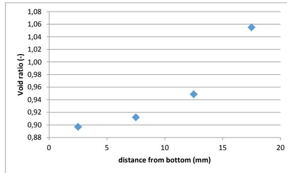
**Figure 3-4** *Distribution of void ratio over specimen height, from bottom end to surface*
