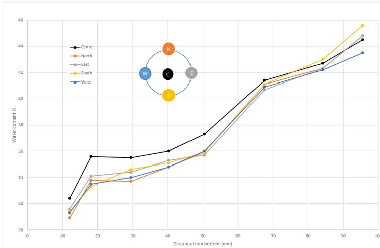
**Figure 5-7** Water content along the vertical at different locations
