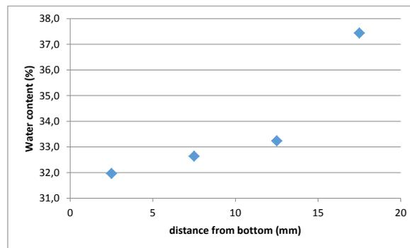
**Figure 3-2** *Distribution of water content over specimen height, from bottom end to surface*
