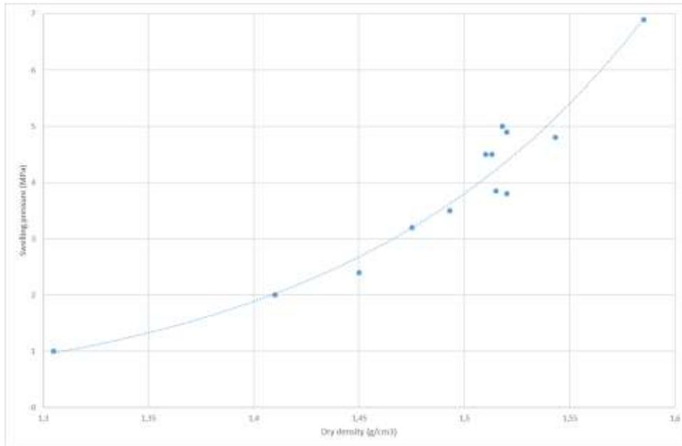
**Figure 4-10** Swelling pressure in function of dry density for FSS mixture type
