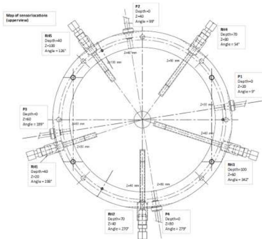
**Figure 4-2** Radial cut of the cell with the location  $z$ ,  $\theta$  of the sensors – RH and Pressure (total)
