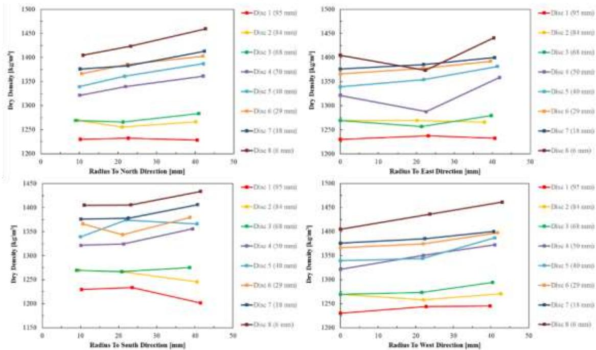
**Figure 5-8** Dry density distributions in the radial directions for block-pellet sample at the end of the test (after 672 days).
