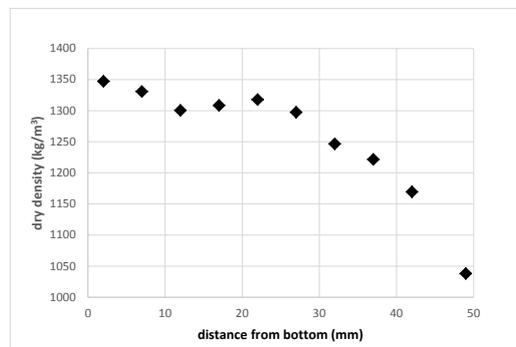
**Figure 3-10** Distribution of dry density over specimen height, from bottom end to surface
