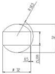
**Figure 4-4** *Geometry of one pellet*
