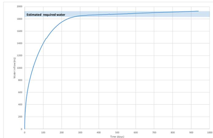
**Figure 4-9** *Water inflow during the test*
