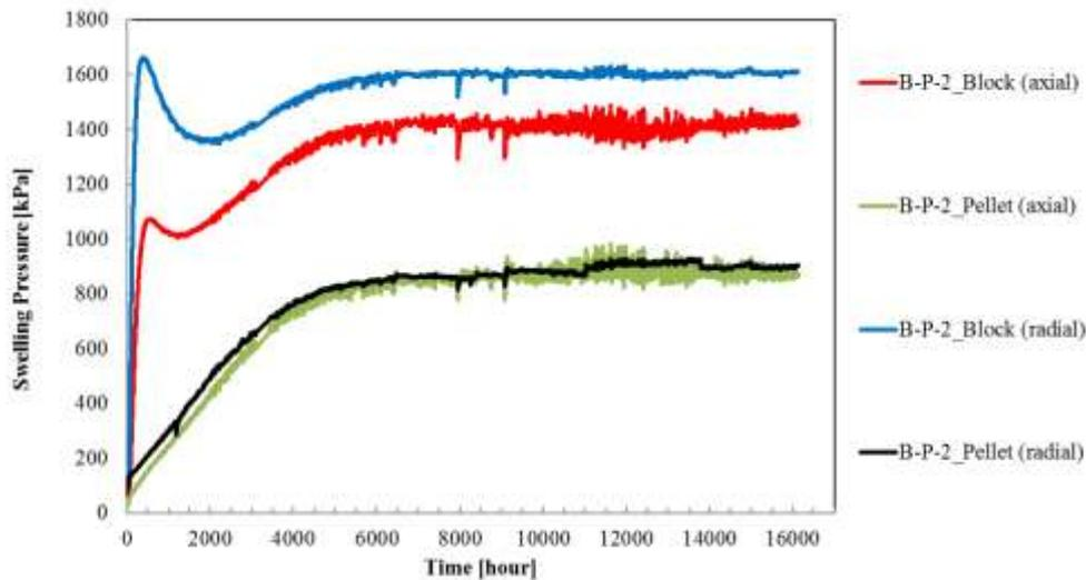
Figure 5-4 Swelling pressure in radial and axial directions function of time
