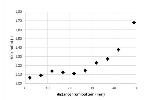
**Figure 3-11** Distribution of void ratio over specimen height, from bottom end to surface
