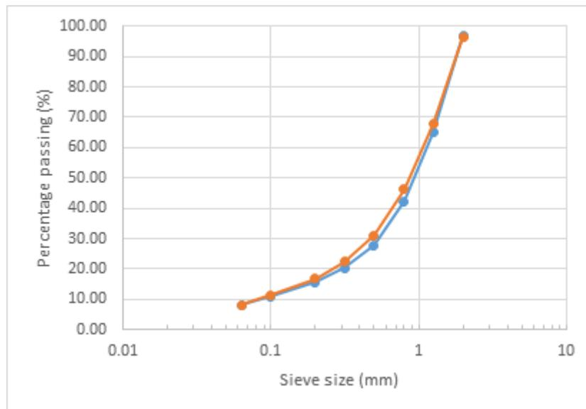
**Figure 4-5** *Grain size distribution for crushed pellets*
