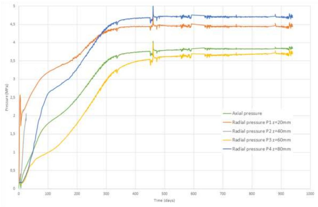
**Figure 4-6** Swelling pressure measured radially and axially
