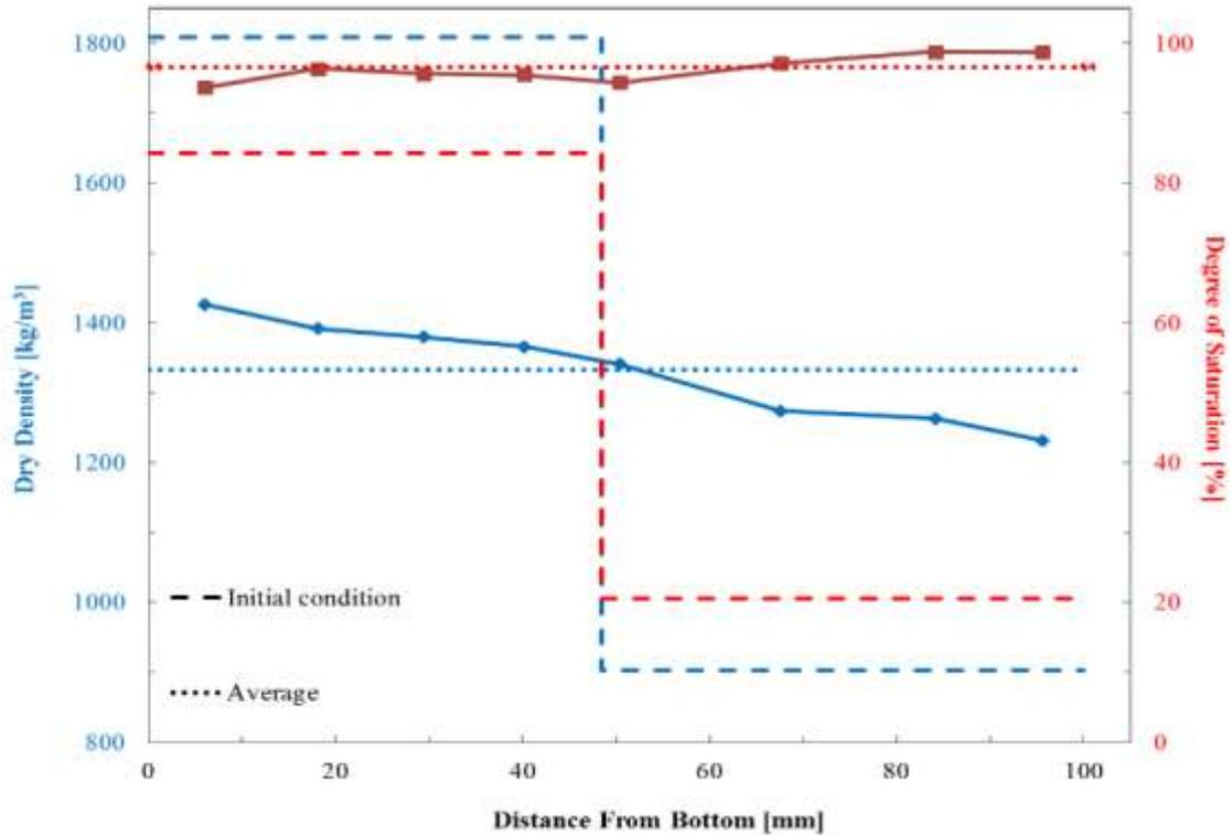
**Figure 5-6** Dry density and degree of saturation distributions over the height of block-pellet sample at the end of the test (after 672 days). Blue diamonds and red squares represent averaged dry density and degree of saturation values, respectively on each height at the end of the test. Dashed and dotted lines represent initial, unsaturated condition and average values over sample volume at the end test, respectively.
