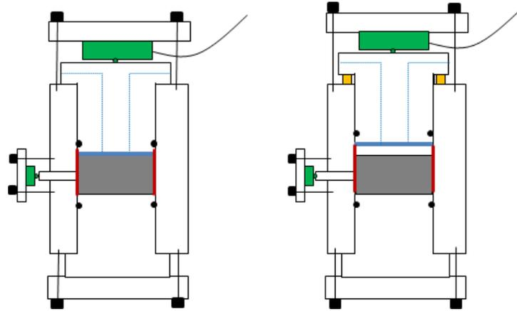
**Figure 3-1** *Set-up used for the axial swelling tests. The red lines represent the lubricated surfaces and the blue lines represent filters and water supply. The radial pressure transducer is placed 10 mm from the bottom end of the specimen*
