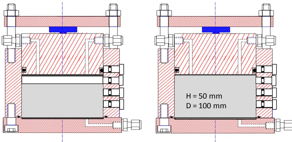
**Figure 3-8** Set-up used for the axial swelling tests. Water is only supplied from a filter placed above the specimen
