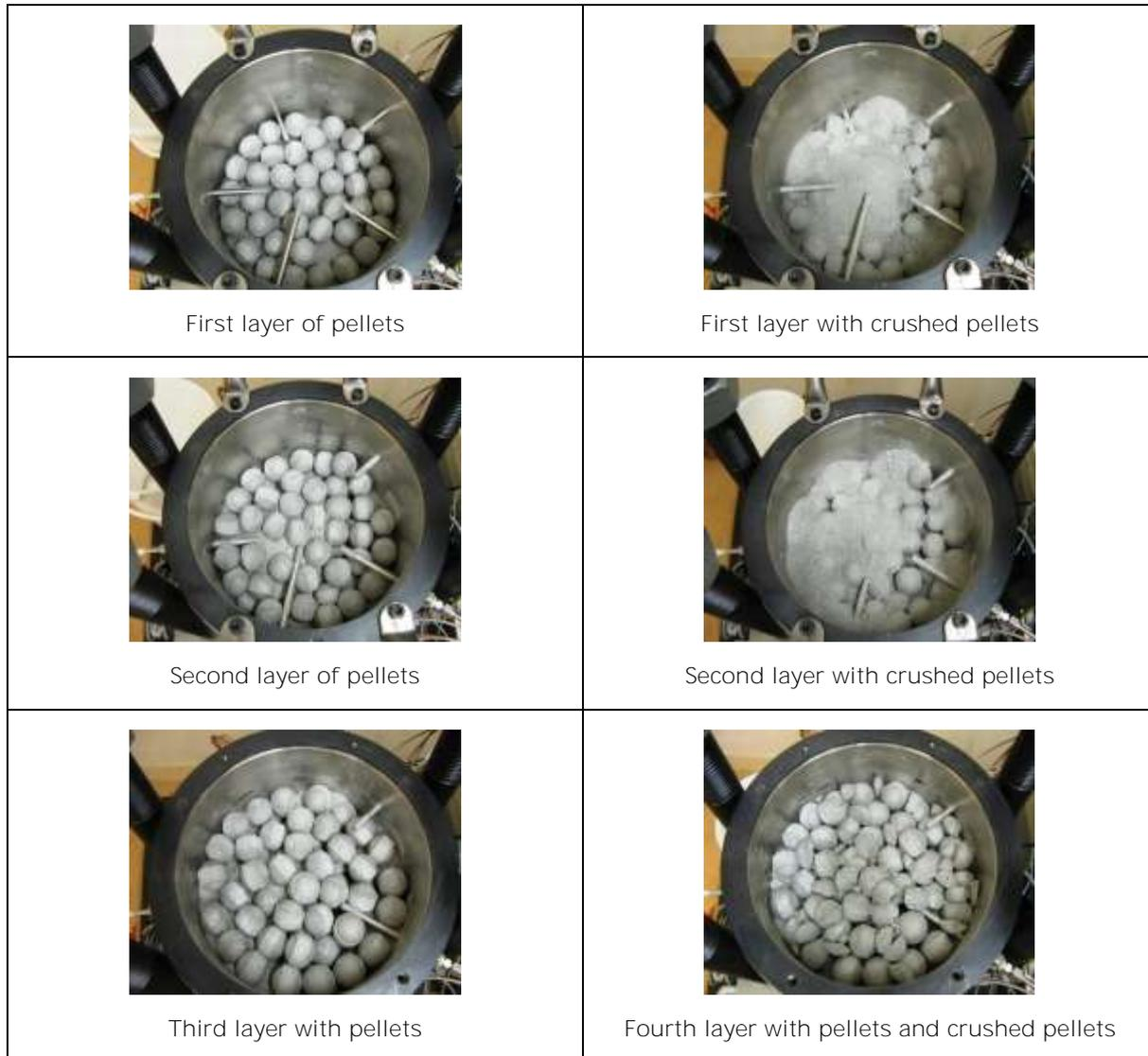
**Figure 4-3** *Installation of the material in the cell – layer by layer*
