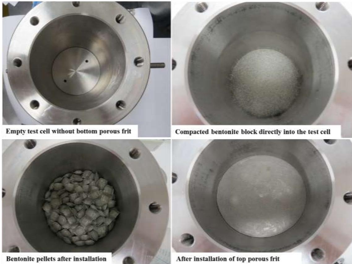
**Figure 5-3** Pictures of the installation of the block-pellet test
