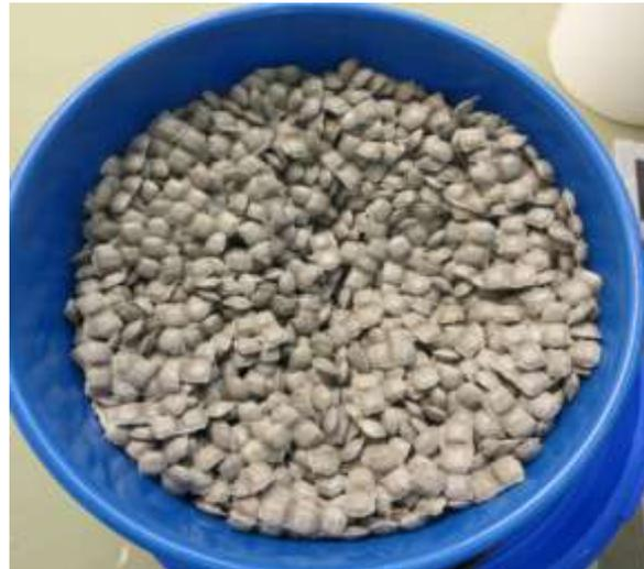
**Figure 5-2** *Picture of MX-80 pillow-shaped pellets as received before sieving.*
