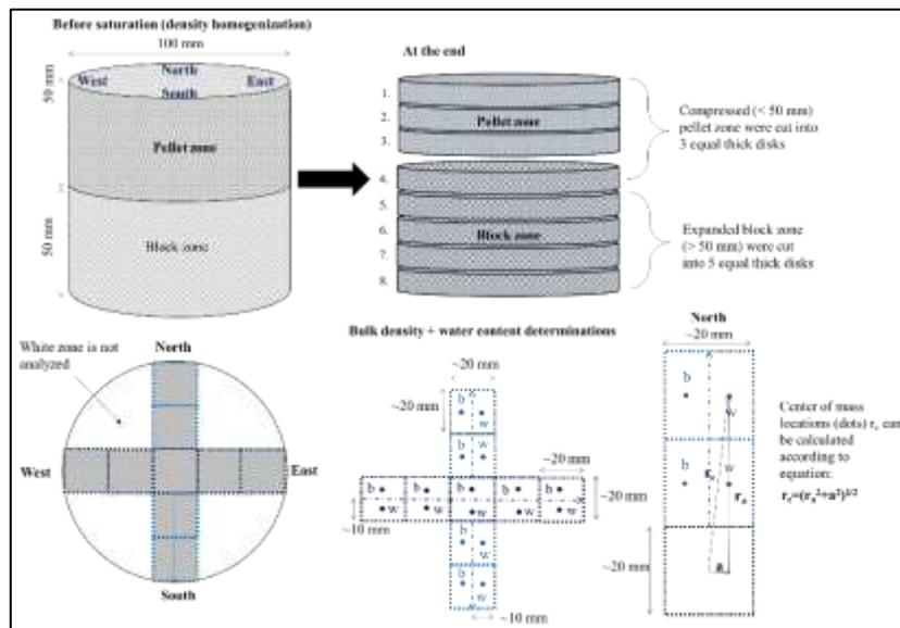
Figure 5-5 Post-mortem sectioning layouts for water content and bulk density determinations. Block and pellets zones were cut into eight equal thick disks, each disk was cut into nine squares (center + 2 squares per north, east, south and west directions) and each square was cut into halves for bulk density (b) and water content (w) determinations.
