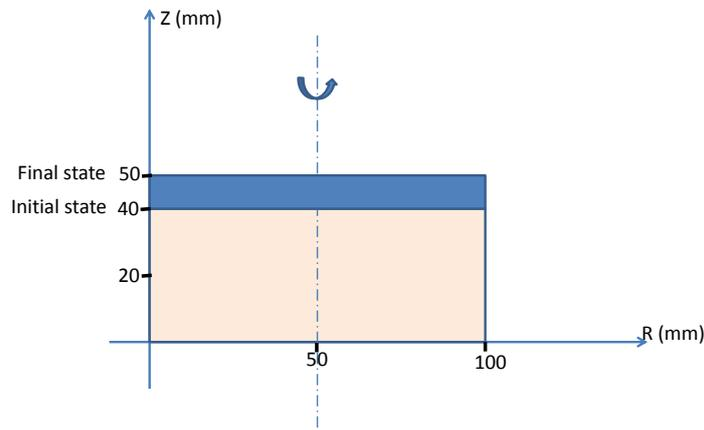
**Figure 3-14** Schematic 2D-representation of the bentonite plug
