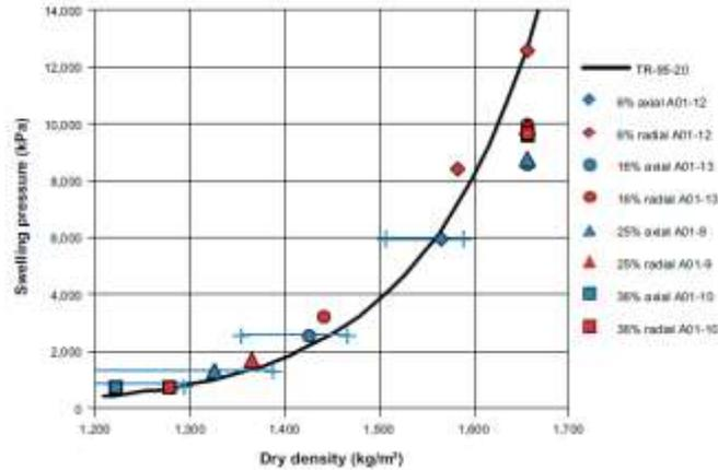
**Figure 3-6** Measured axial and radial stresses (A01-13 on graph) after first saturation and after the second stage of the test. Results from other tests from (Dueck et al. 2011, and 2014).
