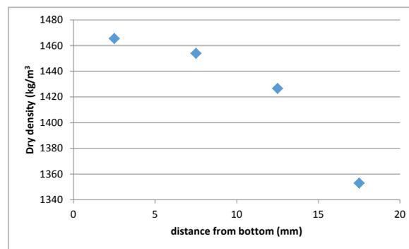
**Figure 3-3** *Distribution of dry density over specimen height, from bottom end to surface*
