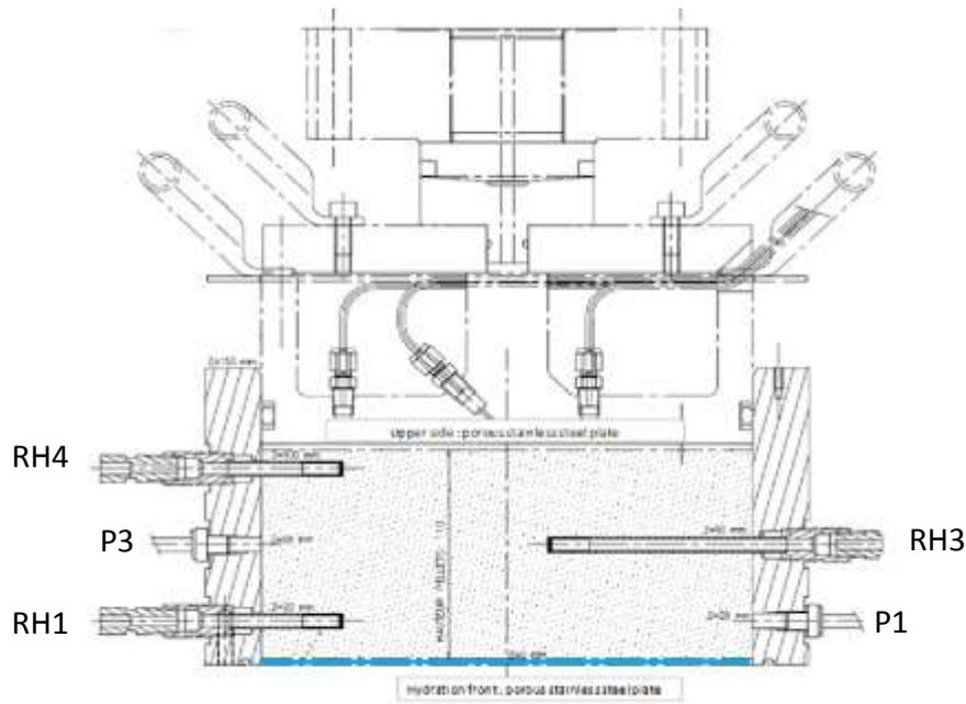
**Figure 4-1** Vertical cut of the cell – water is supplied by a filter above the specimen
