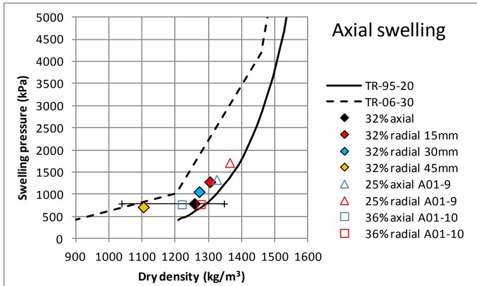
**Figure 3-13** Swelling pressure plotted as a function of dry density. The radially measured pressures are plotted with the dry density measured at the corresponding locations. Axially measured pressure is plotted with the average dry density. Also shown are results from the previous tests
