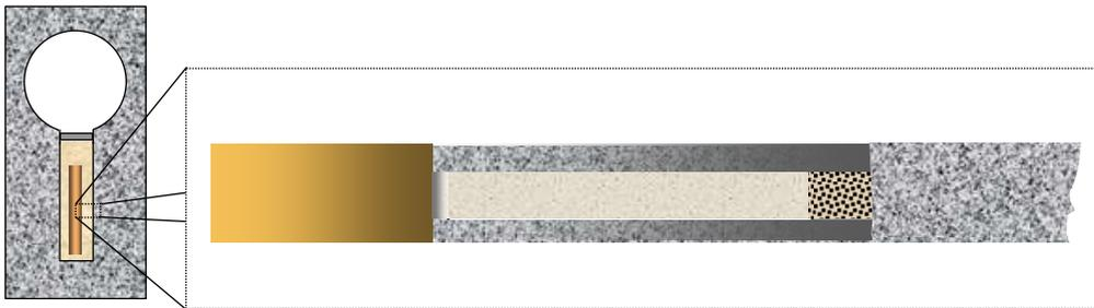
Figure 4-17 A schematic drawing of the CRT geometry and a blow up of a disc at the mid-section.
