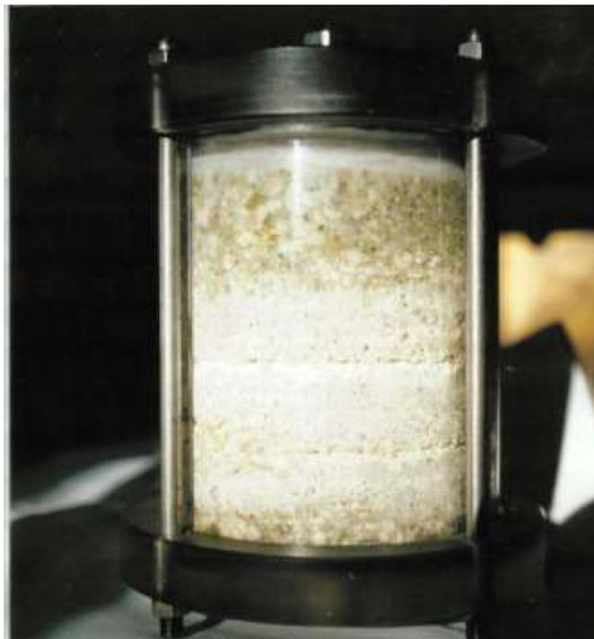
*Figure 1-32 Perspex cell used in joint sealing tests*
