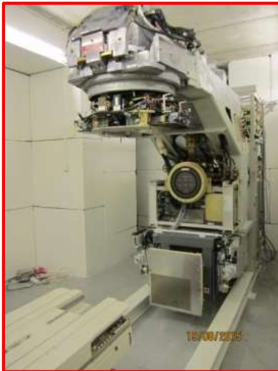
Linac X-ray source, 6-20 MeV
