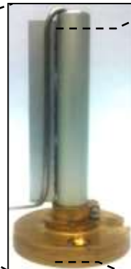
Sample holder (aluminum tube)
