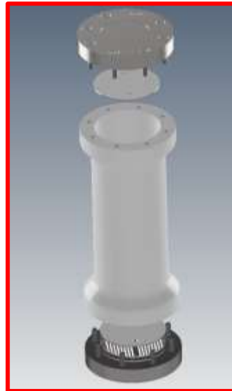
Sample chamber design -Diameter 100 mm.
