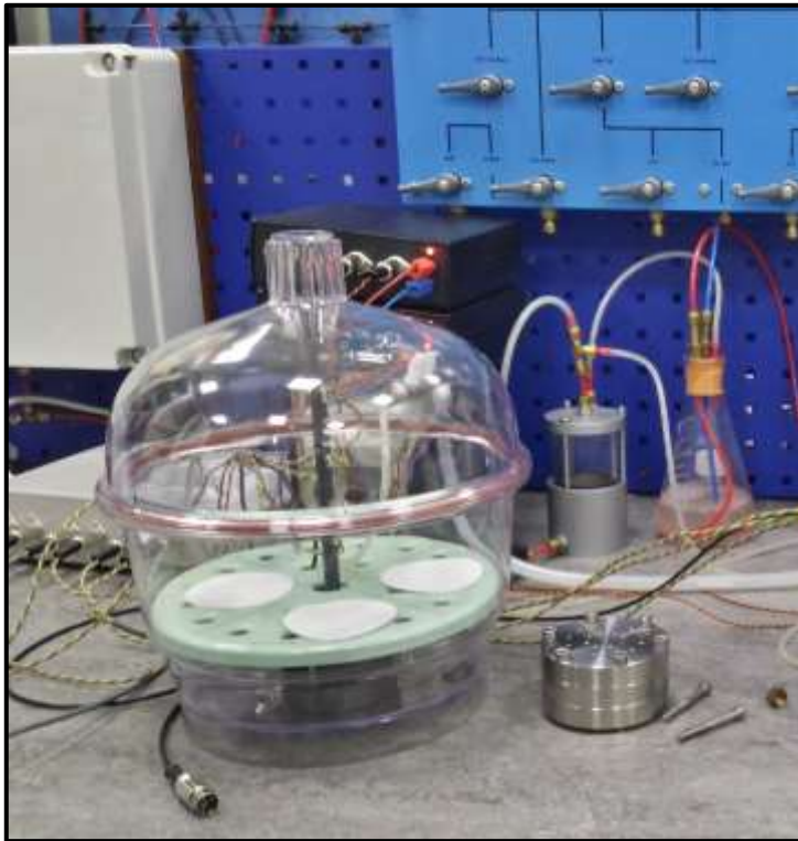
Desiccator with Relative Humidity (RH) suction control
