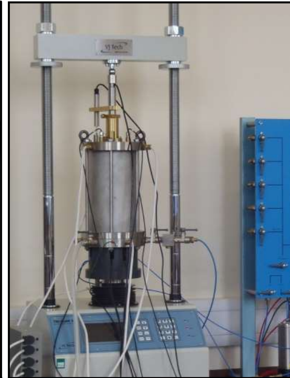
Temperature and suction controlled triaxial cell
