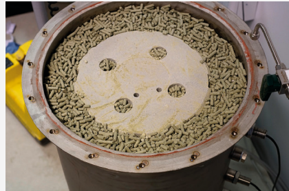
Experimental set up with a bentonite block and extruded bentonite pellets around it. © SKB
