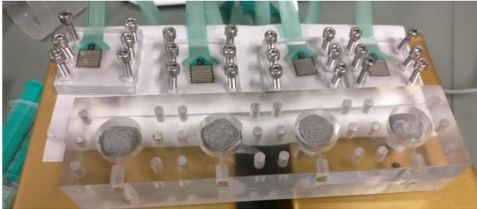
**Figure 4-67. Preliminary test cell array with bentonite pellet samples. The cells are still open and the pressure sensors can be found above the sample cells**
