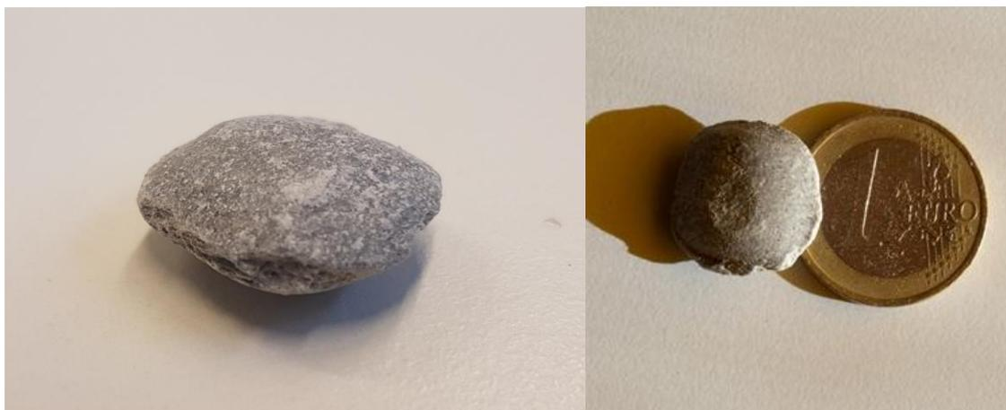
**Figure 4-66. MX-80 pellet used in the tests**
