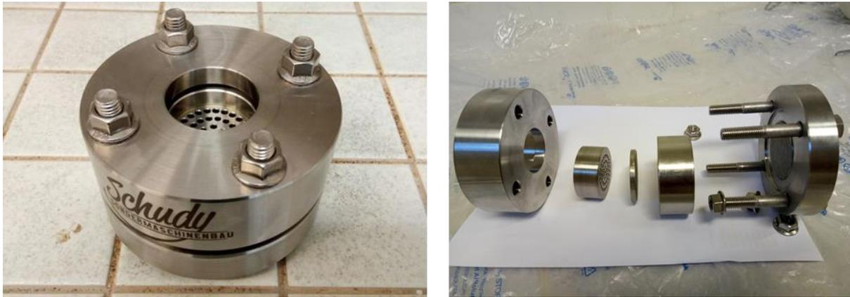
**Figure 3-25. Constant volume cells for measurement of retention curves**
