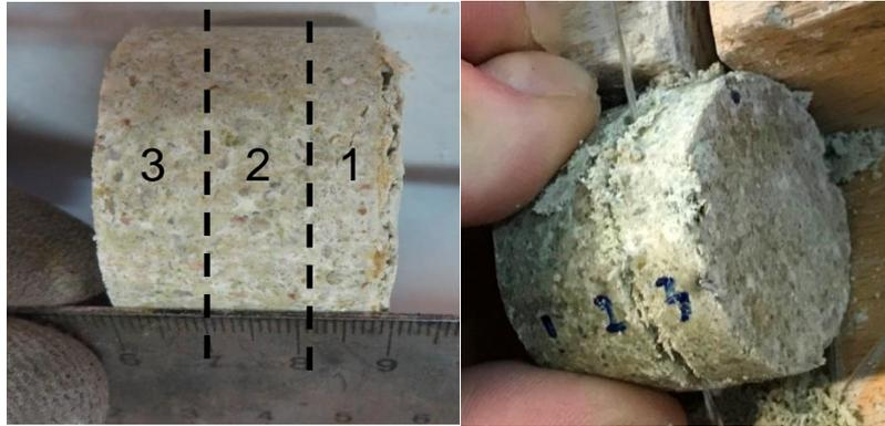
**Figure 4-27. Final subsampling after extraction of samples from the GAP tests cells**
