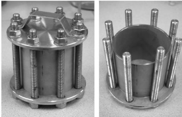
**Figure 4-57. Small scale experiment vessels**
