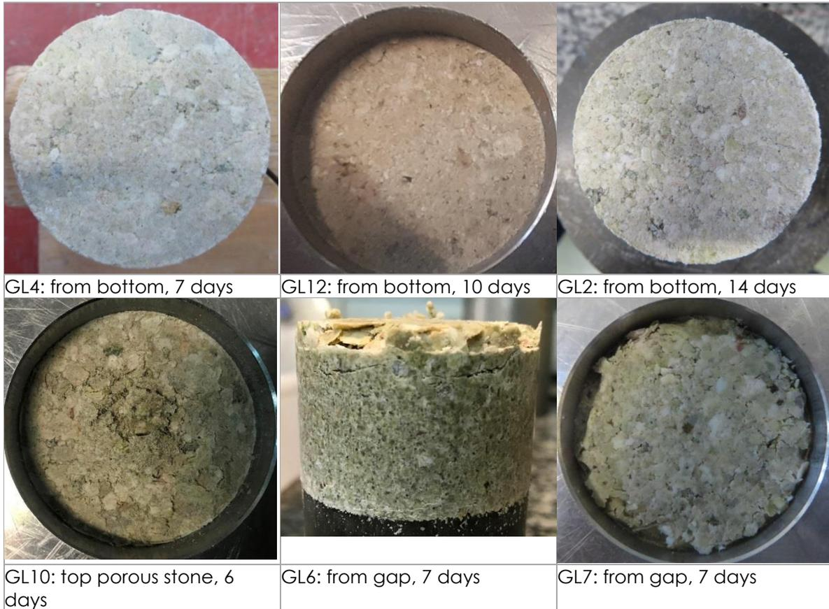
**Figure 4-53. Appearance upon dismantling of some of the shorter GAP-liquid tests (hydration from bottom or gap)**
