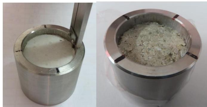
**Figure 4-24. Intermediate measurement of gap height in GAP-vapour tests**
