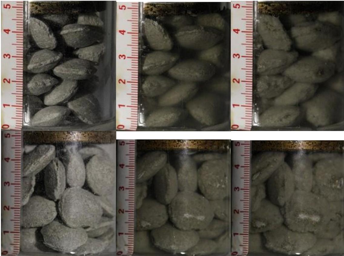
**Figure 4-79. Pellet cluster in the acrylic glass tube; pre-tests 1 & 2 after 0, 1, and 10 min**
