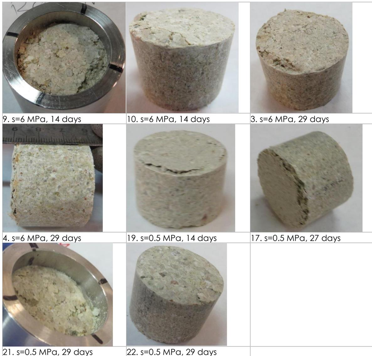
**Figure 4-38. Appearance upon dismantling of some of the shorter GAP-vapour tests**
