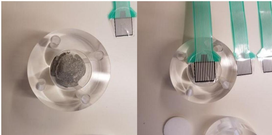
**Figure 4-69. Single pellet emplaced in the cell, bedded on pellet fragments (left). Faced down, the pressure sensitive foil is placed onto the bentonite material (right)**
