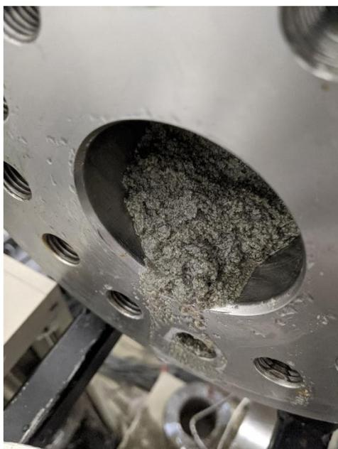
**Figure 4-15.** During decommissioning of Test 16 (3M NaCl), the clay was found to still be in a fluid state at the end of the vessel which original contained only water. [BGS (C) UKRI]
