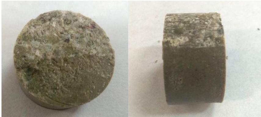
**Figure 5-4. Appearance of the cylindrical sample obtained for gas testing in test CW1**
