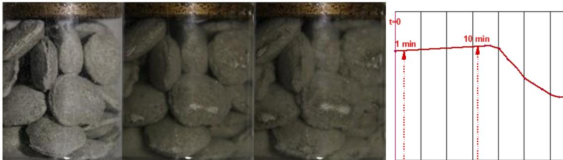
**Figure 4-87. Pellet cluster in the pre-test, after 0, 1, and 10 min and swelling pressure**
