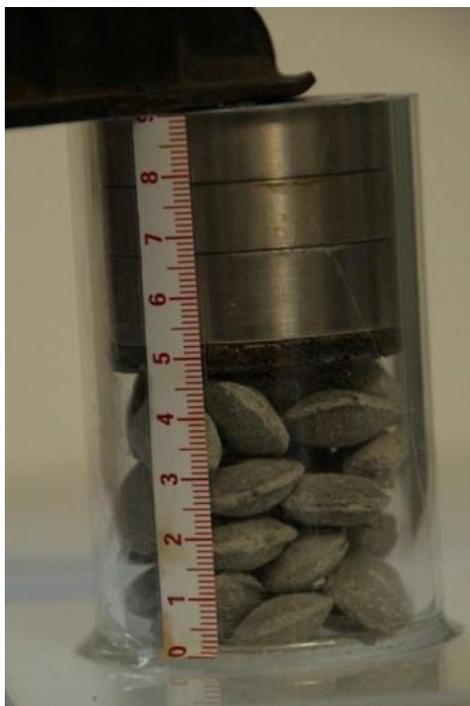
**Figure 4-78. Pellet cluster installed in the acrylic glass tube for pre-test 1, dry at  $t = 0$**
