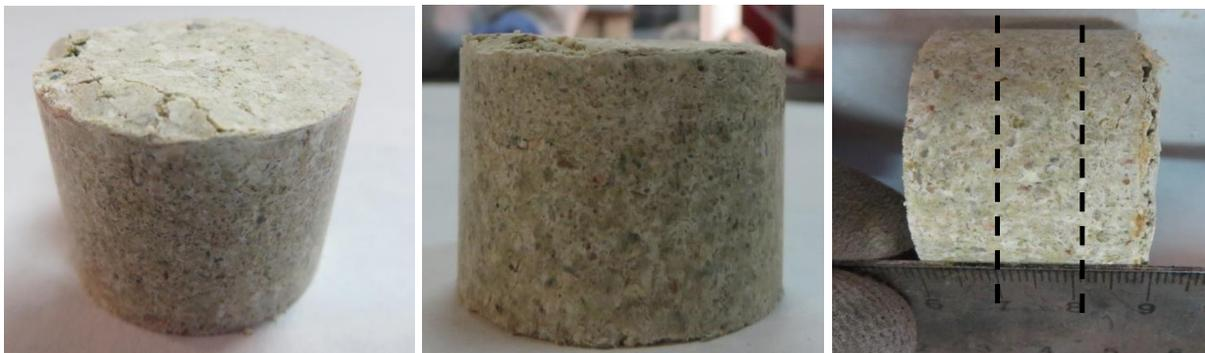
**Figure 4-33: Appearance of samples after extraction of the cells and subsampling for postmortem analyses**
